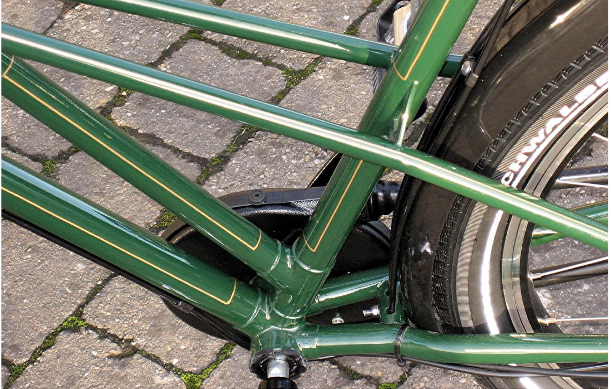
The bottom bracket shell is fully lugged for the bottom tube, seat tube and chainstays and, above it, there is the beautiful lug to join the trapeze "top tube" and the seat tube.
