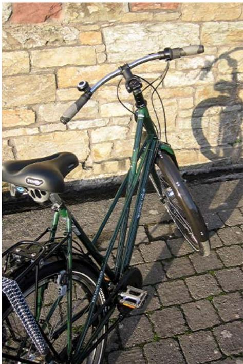
Here the frame crosses are visible where the lateral full-length mixte rails pass the “top tube” and the seat tube. The twin lateral rails are soldered to both the single tubes where they cross them; there are more detailed photographs further down. Those are my favourite pedals, the VP 191. of which a pair arrived with the bike.
