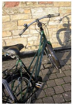
Here the frame crosses are visible where the lateral full-length mixte rails pass the "top tube" and the seat tube. The twin lateral rails are soldered to both the single tubes where they cross them; there are more detailed photographs further down. Those are my favourite pedals, the VP 191. of which a pair arrived with the bike.
